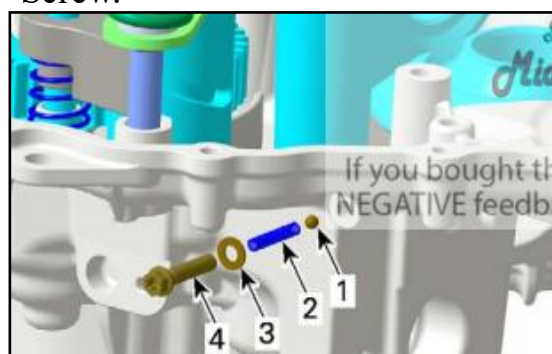
1.Ball 2.Spring 3.Sealing ring 4.screw
